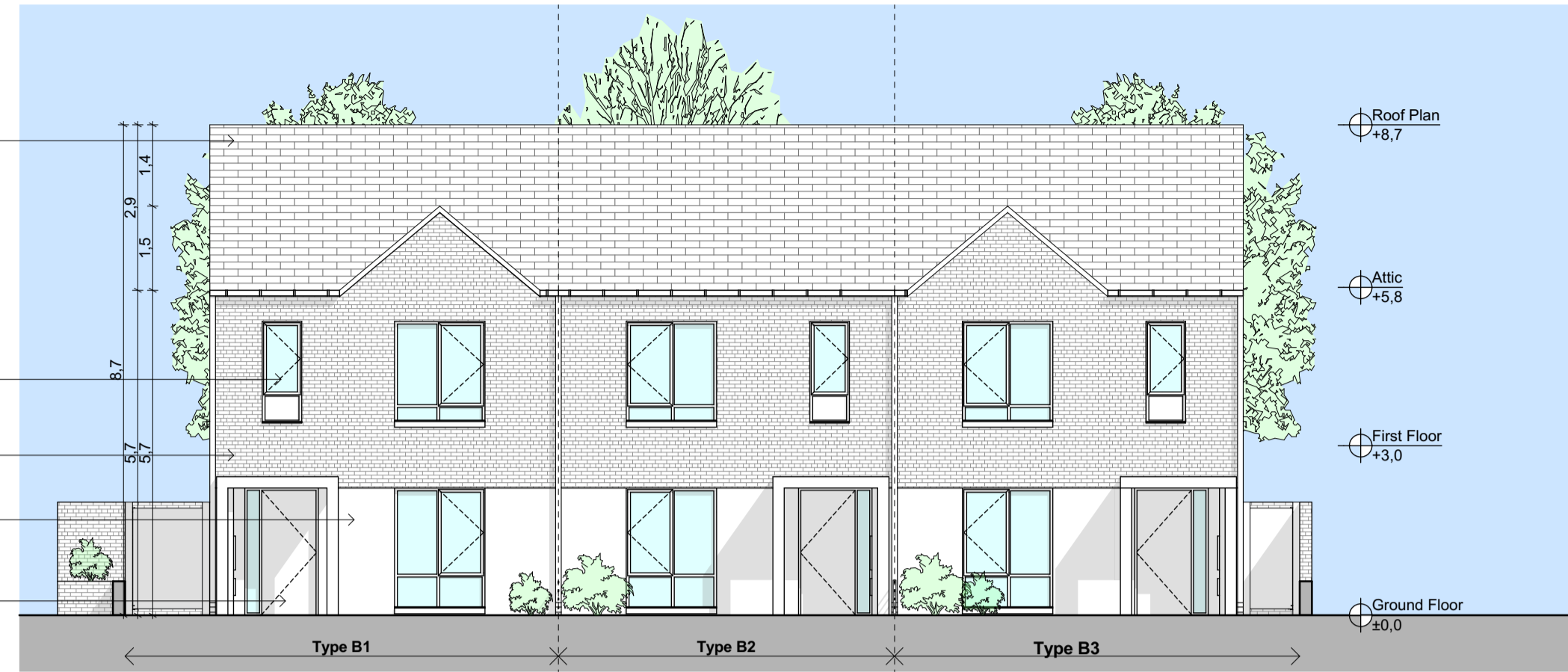
Front Elevation SCALE 1:100
